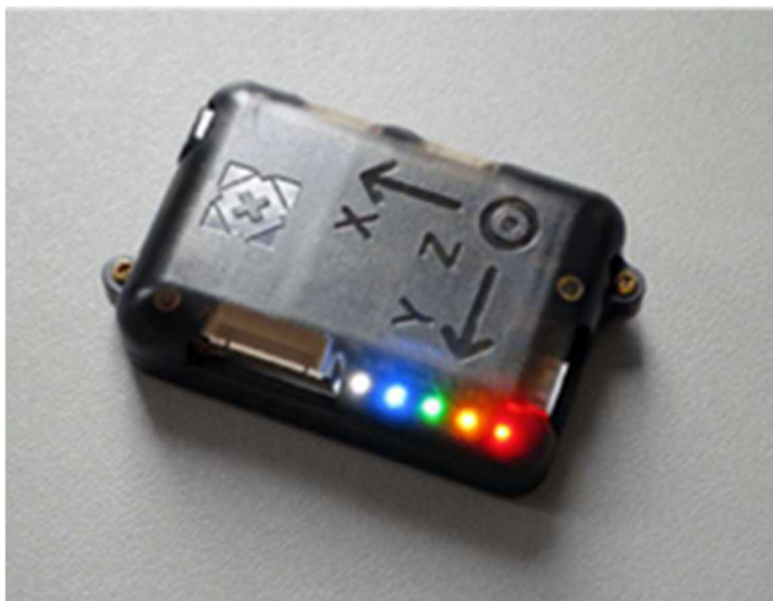
Inertial Measurement Unit (IMU) used by KGHM Cuprum for collecting data in
