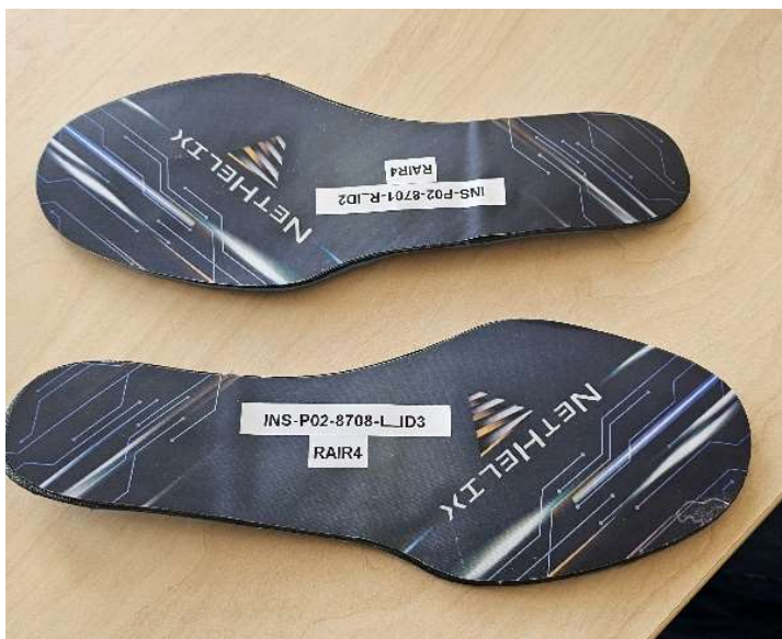
Smart insoles (developed by Cyprus Research & Innovation Center Ltd. – CyRIC) enhancing the health and safety of users in mine operational environment through embedded sensors that monitor foot activity (e.g., walking, stair ascending/descending, etc.) and provide alerts for several events (e.g., unconscious, injured or over-tired users).
